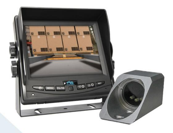
This new camera system was designed specifically with forklifts in mind. The RVS-77F6033 will hasten every job in which forklifts are involved. The system includes a 5.6" LCD monitor and a heavy duty camera with an IP69K waterproof rating, as well as all the components required for a quick and simple installation. The camera is easily mounted to the fork in minutes.
