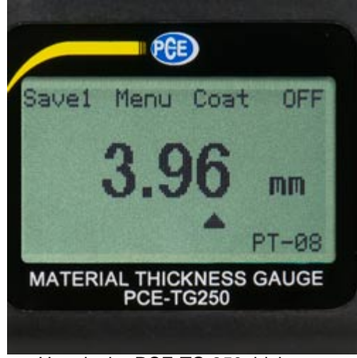
Here is the PCE-TG 250 thickness gauge being used.
