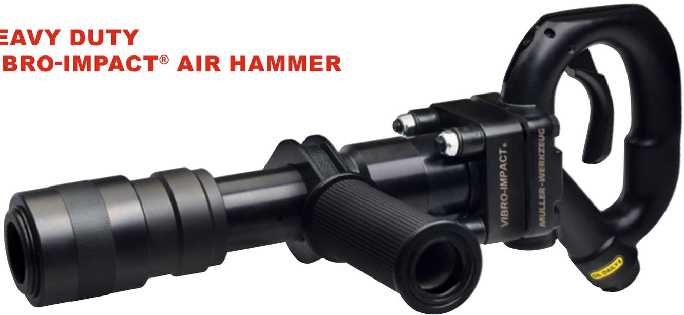
Heavy duty **VIBRO-IMPACT®** air hammer to loosen tight connections on trucks, agricultural and construction vehicles, etc. The high performance air hammer helps to disassemble e. g. conical seat connections, wheel bearings, bushings, rusted screw connections. Can support pullers as well.
