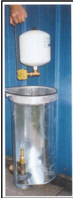
Lifting with Pull Strap Steel Casing
