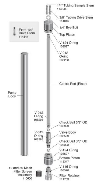
(Filter Retainer and Screen Assembly (Complete) 110517)
