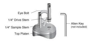
**Note:** When required, use a small (2 mm) Allen key through the hole to help loosen and tighten the tubing stems.
