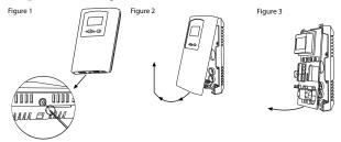
The cover is hooked to the base at the top edge and must be removed from the bottom edge first. Use a small Phillips screwdriver to loosen the security screw as shown in Figure 1. Use the screwdriver to carefully pry each bottom corner if necessary. Tip the cover away from the base and sit it aside as shown in Figure 2.
