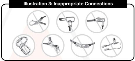
**NOTE:** Other than 3,600 lb. (16 kN) gated hooks, large throat opening snap hooks should not be connected to standard size D-rings or similar objects which will result in a load on the gate if the hook or D-ring twists or rotates. Large throat snap hooks are designed for use on fixed structural elements such as rebar or cross members that are not shaped in a way that can capture the gate of the hook.
