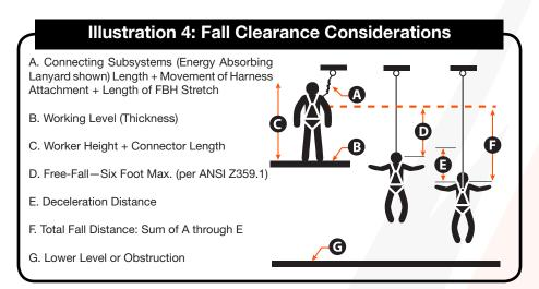
If there is a risk of a fall or if the only anchorage point is below the attachment points on the harness, it is essential to use a lanyard provided with an energy absorber. Before using a shock absorbing lanyard, ensure that there is sufficient fall clearance below the user to prevent any collision with the structure or ground.
